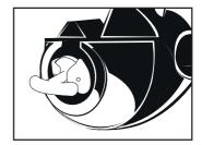
Rotate the tool around the curl chamber to remove any build-up of
