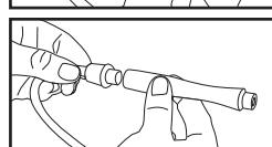
4. Connect the end of the tube to the hand-held device.
