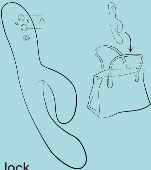
**EN** To activate the Travel Lock feature, hold the plus and minus buttons for 3 seconds, the device will pulsate and your device will 'lock'. To disable Travel Lock, press the buttons again for 3 seconds or charge your device. Nova will pulse and your device will "unlock".
