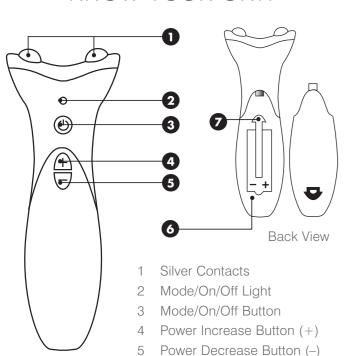
Battery CompartmentBattery Release Tab
