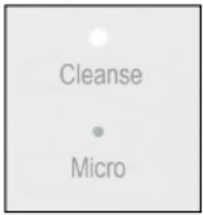
The Treatment & Charging Indicator lights will continuously cycle during charging.
