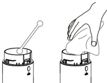
3. Use a clean swab or cloth to clean the unit. Please ensure no dust or dirt is obstructing the air inlet on the base of the unit.
