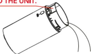
2. Empty water via the water drainage side, opposite the air inlet.
