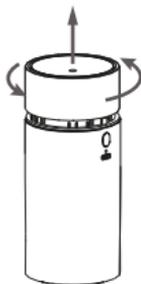
1. Twist the cover anti-clockwise (to the right) to remove.
