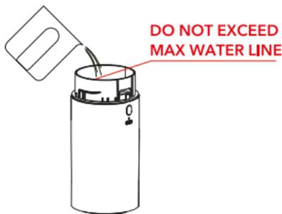
2. Add water to the water tank with a suitable measuring cup until the water reaches the max. water level line.
