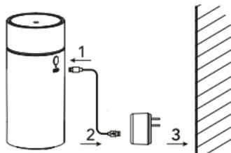
2. Once connected properly the indication light will turn red to indicate that the unit is being charged.
