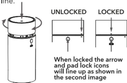
4. Replace the cover by twisting clockwise (to the left) to secure the lid in place.
