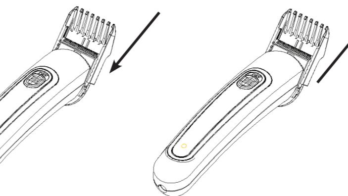
Reset the blades, and press the full parts until hearing the "KA" sound.
