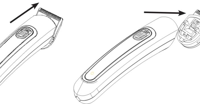
Using brush to clean the blades parts, and lubricating the space between the stationary and moving blades with 2 or 3 drops of oil after every few uses.
