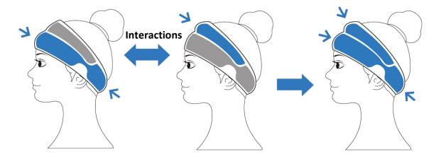
Massage program: **ACUPRESSURE** - compression movements of the upper and lower air bag simultaneously. Imitates finger movements around the entire circumference of the head.
