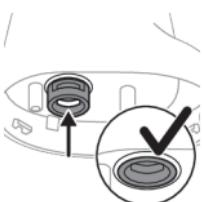
**8** Push the nozzle retention ring into the device. The nozzle retention ring should be fully flushed with the body.
