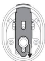
**6** Remove the nozzle release button slider.
