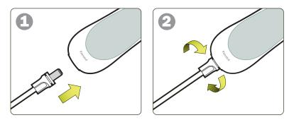
**Step 1:** Connect the power cord to the device. **Step 2:** Turn the connector one quarter turn until it locks in place.
